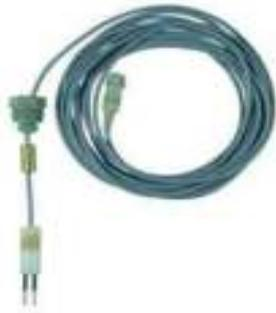
The supplied conductivity Level Probe is used as a minimum water level detector in the rainwater tank. The standard length of cable supplied is 15m. This can be extended to order, up to 100m. It carries a very low voltage/current.
